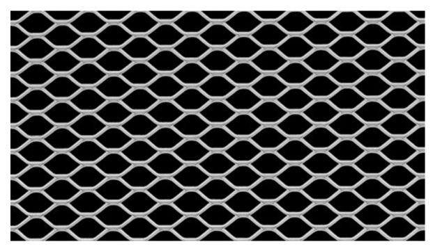
LW Pitch:19.05mmStrand Width:1.22mmSW Pitch:9.50mmThickness:1.20mmWeight:2.41 kg / m2Open Area:74%
